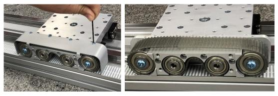
7.3 Next remove the screws securing the drive assembly to the base block assembly. Set the screws aside.
