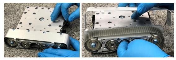
7.15 Remove the old endless belt and substitute it with a new replacement. **NOTE:** Remember to add a small amount of CRC 03055 Food Grade Chain Lubricant to the smooth side (backside) of the endless belt.
