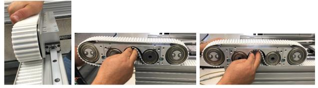
8.16 With the drive assembly/base block assembly fully re-mounted on the stage, insert .004" shims under the idler bearings.
