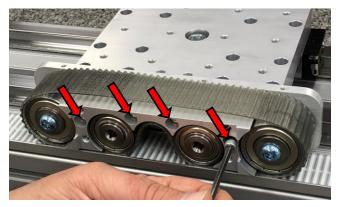
7.4 You can now lift the drive assembly up off of the belt tray. Remove the old endless belt and substitute it with a new replacement. **NOTE:** Remember to add a small amount of CRC 03055 Food Grade Chain Lubricant to the smooth side (backside) of the endless belt.
