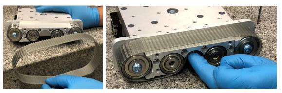
7.16 Install the replacement Endless Belt and press up with your finger in the pinion gap to create tension on the belt. While keeping that belt tension, re-install the Belt Cover with the 4 screws.
