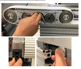
8.14 With the drive assembly now removed from the stage, you can remove the old endless belt and substitute it with a new replacement.
