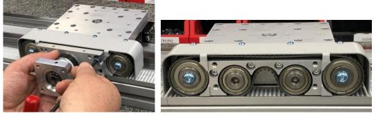
7.2 Next remove the belt cover screws. Set the belt cover and screws aside.
