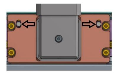
5.2 Now with the belt tensioning set screws still backed off and the dowel pins in the centered slot position, snug up the four mount plate screws completely, then back them off ¼ turn. Next tighten the two belt tensioning set screws all the way, then back them off again. Begin the belt tensioning in the next step.
