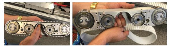
8.5 Re-place the drive assembly onto the belt tray. <u>IMPORTANT:</u> Be sure to keep belt tension by pressing up on the belt within the pinion gap of the drive assembly during the re-install. Use the key on the back of the drive assembly to align with the slot on the base block assembly.
