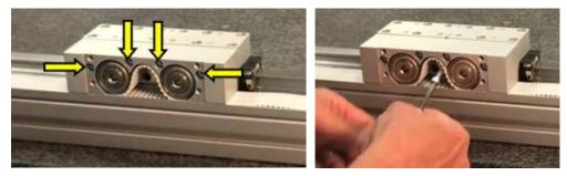
6.12 Now insert .004" shims under the idler bearings, then tighten the mounting screws based on Section 2 Table 2 specifications for the stage assembly model.
