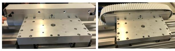
8.3 Next remove the screws securing the drive assembly to the base block assembly, including the hidden, captured screws within the idler stud. Set the screws aside.
