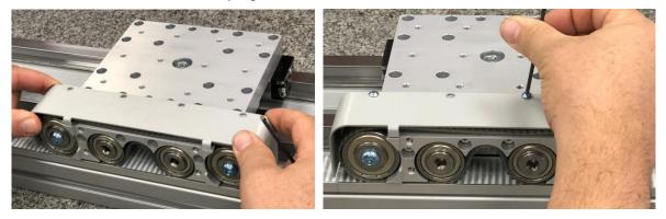
7.9 Re-attach the motor mount plate/motor to the drive assembly. Fasten the screws just snug, then back off <sup>1</sup>/<sub>4</sub> turn.
