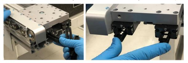
7.14 Next remove the belt cover screws. Set the belt cover and screws aside.
