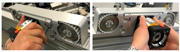
8.12 Next, remove the belt cover screws from the rear of the belt cover. Set the belt cover and screws aside.
