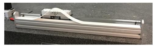
6.10 Re-install the drive assembly onto the belt tray by aligning the drive assembly with the slot on the base block assembly. Be sure to fully insert the belt loop into the pinion gap of the drive assembly as you perform the re-install.
