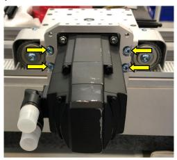
7.12 Next, remove one of the hard stops (and End Cap if present) to allow the drive assembly and attached base block assembly to be removed from the stage.
