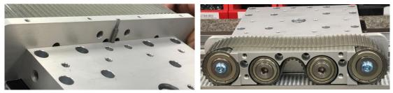
7.6 Re-attach the screws securing the drive assembly to the base block assembly. Fasten the screws just snug, then back off <sup>1</sup>/<sub>4</sub> turn.
