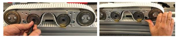
8.8 When the screws are fully tightened, remove the shims and re-attach the belt cover.
