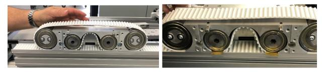
8.17 Now tighten the drive assembly screws per Section 2 Table 2. After fully tightening the screws you can remove the shims.
