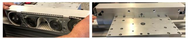
8.9 Re-attach the motor mount plate/motor to the drive assembly. Fasten the screws just snug, then back off <sup>1</sup>/<sub>4</sub> turn.
