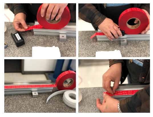
9.6 When you are ready to re-install or replace the lower 'static' belt, remove the backing from the 3M VHB Tape to expose the adhesive. You can use a razor blade to separate the backing from the tape.
