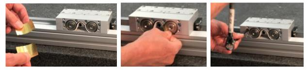
6.13 Re-attach the motor mount plate/motor to the drive assembly. Fasten the screws just snug, then back off ¼ turn.
