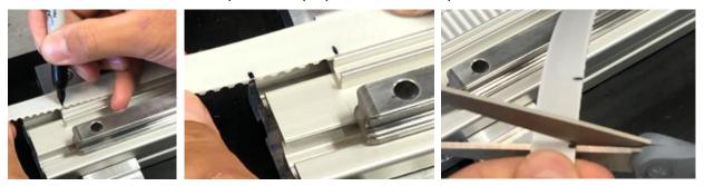
6.8 Before returning the trimmed upper belt to the belt tray, check the lower belt to ensure lubrication is present. If dry, apply a small amount of CRC 03055 Food Grade Chain Lubricant to the lower belt. You can now lay the trimmed upper belt back onto the lower belt (as shown) with both belt edges flush to the ends of the belt tray.
