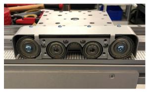
7.13 While keeping the belt tensioned by hand within the pinion gap of the drive assembly, you will roll the drive assembly off of the stage.
