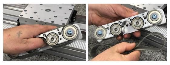
7.5 Re-install the drive assembly on the belt tray. <u>IMPORTANT:</u> Keep the endless belt tensioned by pressing up on the belt within the pinion gap of the drive assembly. Align the key on the rear of the drive assembly with the slot on the drive block to assist with the re-installation.
