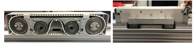
8.19 Re-attach the motor mount plate/motor to the drive assembly. Fasten the screws just snug, then back off ¼ turn.
