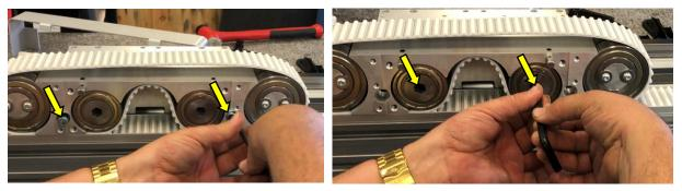
8.4 You can now lift the drive assembly off of the belt tray. Remove the old endless belt and substitute it with a new replacement.
