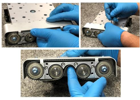
7.17 Now slide the drive assembly and attached base block assembly back onto the stage while keeping belt tension throughout. The bearing rails will cause the plastic bearing ball retainers (Arbors) to be pushed out of the bearing blocks.
