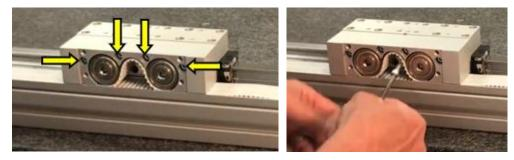
6.3 Once the screws are removed – lift the drive assembly off of the belt tray. Note: The rear of the drive assembly is keyed to mate with the slot on the drive block assembly.
