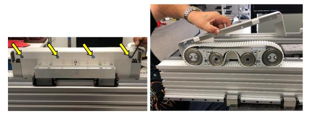
8.13 While keeping the belt tensioned by hand within the pinion gap of the drive assembly (as shown below), you will roll the drive assembly off of the belt tray. <u>IMPORTANT</u>: As you roll the drive assembly off, be sure you have the necessary number of plastic ball bearing retainers (aka Arbors) available to slide into the bearing blocks <u>as they come off of the bearing rails</u>.
