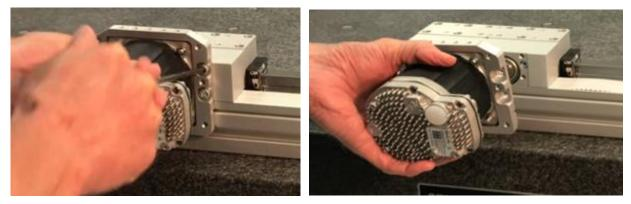
6.2 Next remove the screws that secure the drive assembly to the base block assembly. (Be advised - some configurations may have two screws inside the pinion gap of the drive assembly, as shown).
