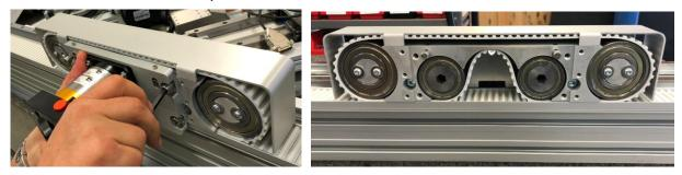
8.2 Next remove the belt cover screws. Set the belt cover and screws aside.
