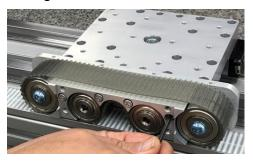
7.7 Insert .004" shims under the idler bearings, then finish tightening the drive assembly mounting screws per Section 2 Table 2.
