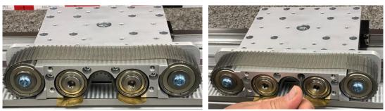
7.8 When the screws are fully tightened, remove the shims and re-attach the belt cover.
